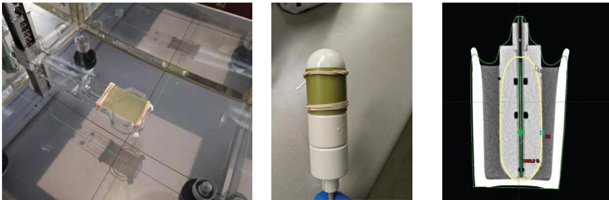
FIGURE 1 Film set-up for the 6 MV and Ir-192 calibrations. (a) Shows the film set-up for the 6 MV calibration. The precut film was fixed on top of a Roos chamber holder attached to an MP1 phantom tank. (b) and (c) illustrate the Ir-192 calibration. The precut film piece was wrapped around and fixed to a cylinder high dose rate (HDR) applicator of 40mm in diameter. (c) The setup was scanned, and a treatment plan was prepared for calibration with the Ir-192 source
